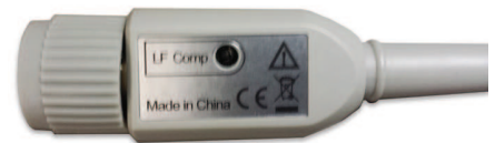
Figure 2. Low-frequency compensation adjustment (for N2840A/41A/42A/43A/53A)
