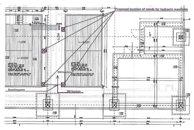
2. The movable part of the high-pressure oil distribution system comprises high-pressure line and return hoses and threaded connectors for the start/stop valves of the manifold and the electrohydraulic cylinders. The scope of delivery also includes protective flexible sleeves for high-pressure as well return lines and a set of connectors and fittings for connecting and routing these hoses to the electrohydraulic cylinders.
